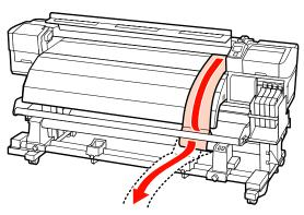
Bring the adjustment paper to a position 5 cm from the left edge of the roll core. Pass the lead edge of the adjustment paper by the front of the media guide bar and then insert it into the printer.
