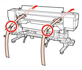
As shown in the illustration, align Hole 1 of film b with the screws on the left and right edges of the loading guide, and then adhere it.
