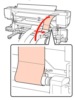
At the front side of the printer, keep the adjustment paper taut, place a ruler on the front side of the white line on the platen, and then draw a line with a pen or other writing instrument.
