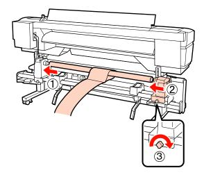
Rotate the handle until part A in the illustration below is fully inserted.
