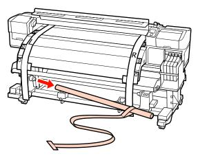
Remove film a from the roll core.
