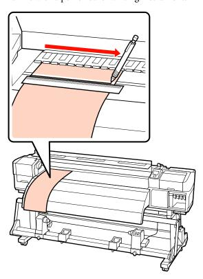
Pull out the adjustment paper from the rear side, move it to a position 5 cm from the left edge of the roll core, and then insert it into the printer.
