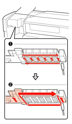
Ink spatters on the base of the print head can be removed using a clean room wiper (available in the market).
