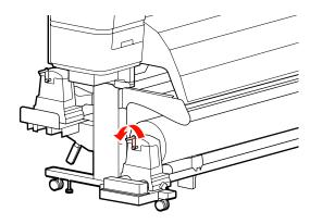
To prevent the media from sliding off the roll, support the roll at its left end.
