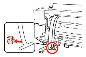
Pull out film a from the printer. Next, loosen the right roll core holder locking screw and remove the roll core holder from the roll.
