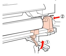
To ensure the roll holder is inserted into the roll core sufficiently, push the center section on the side of the roll holder towards the roll end twice.
