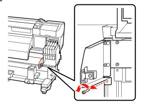
Use a hexagon wrench (large) to remove two screws.
