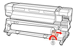
Lower the roll onto the roll support.
