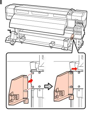
Use the hexagon wrench (large) to tighten and firmly secure the two screws that were provisionally secured.
