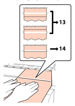
While checking the state of the two lines on the front side of the printer, use the hexagon wrench to adjust the screw on the rear side of the printer so that the drawn line aligns with the position of the dotted line.
