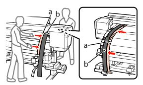
Attach a counterweight to film a. After film a stops swinging, record the value of the scale on the front side of the white line of the platen.
