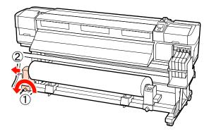
Lower the roll onto the roll support.
