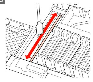
Return the wiper cleaner that was removed in Step 2 to its original position.
