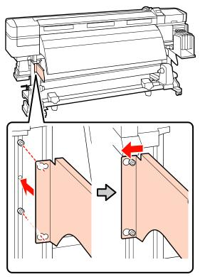
Use the hexagon wrench (large) to tighten and firmly secure the two screws that were provisionally secured.
