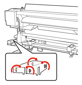
Loosen the roll holder fixing screws and adjust the roll holders so that the distance between the two is wider than the roll core.
