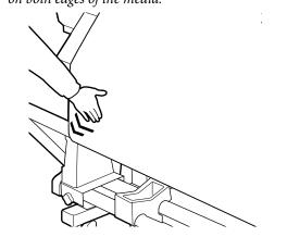
Press the ▼ button to feed the media until the take up roll core begins to turn.
