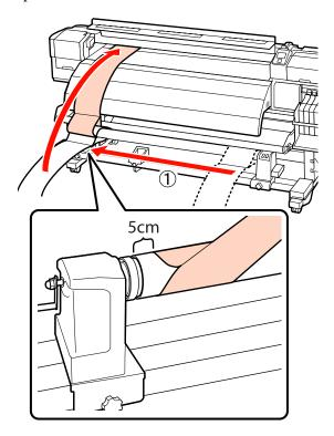
Keep the adjustment paper taut, place a ruler on the front side of the white line on the platen, and then draw a line with a pen or other writing instrument.
