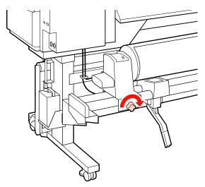
Raise the lift lever on the right side of the printer to lift the media into position, then firmly insert the roll holder.
