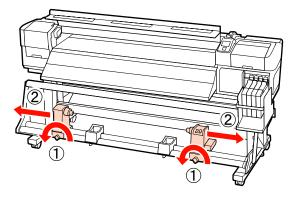
Tighten the roll core holder locking screw to align the right roll core holder with the position of dotted line.
