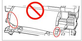
Confirm that the edges of media taken up on the roll core are not misaligned.
