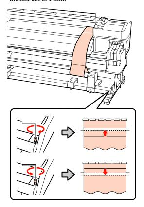
Use the hexagon wrench to tighten and firmly secure the 4 screws.
