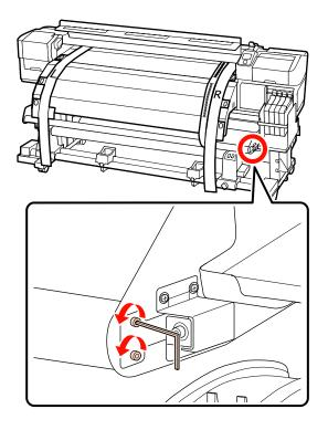
While checking the scale of film a on the front side of the printer, make adjustments using the large hexagon wrench while you use your hand to hold the media guide bar.
