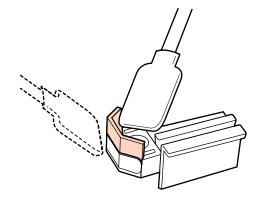
Clean the bottom of the wiper with a cleaning stick.
