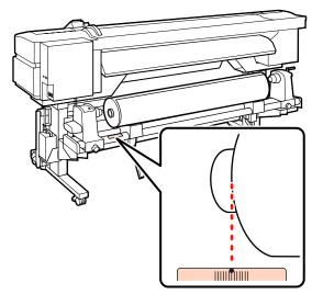
If the label does not have the loading position, mark it on the label as instructed in the *Setup Guide*.
