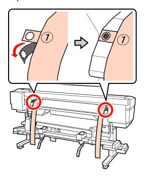
As shown in the illustration, align Hole 2 and 4 of film b at the front of the printer with the screws on the left and right side of the after heater, and then adhere them.
