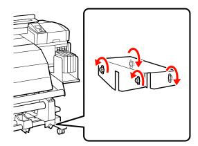
Loosen the roll core holder locking screws and adjust the roll core holders so that the distance between the two is wider than the roll core.
