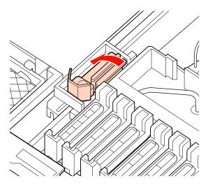
Clean the front and back of the wiper with a cleaning stick.
