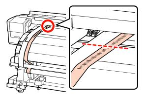
At the front and rear of the printer, raise film a and move it so that it aligns with film b tightly. After film a stops swinging, check the scale where the front side of the white line of the platen passes.
