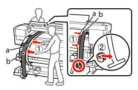
After film a stops swinging, record the value of the scale on the front side of the white line of the platen.
