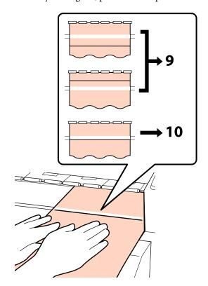
While checking the state of the two lines on the front side of the printer, use the hexagon wrench (large) to adjust the screw so that the drawn line aligns with the position of the dotted line.
