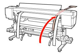
While checking at the front and rear of the printer, align film a with film b tightly.
