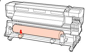
To prevent the media from sliding off the roll, support the roll at its right end.
