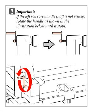
Insert the roll core into the right roll holder. Next, insert the left roll core holder into the roll core, and then tighten the roll core holder locking screw.
