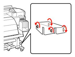
Loosen the roll core holder locking screws and move the left roll core holders to the outside.
