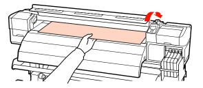
Pull the media straight forward to the leading edge of the after heater.
