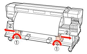
Align the right roll core holder with the right edge of the media and tighten the locking screw.
