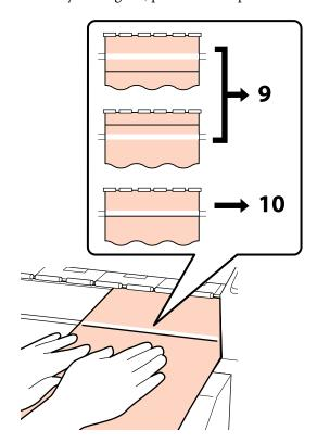
While checking the state of the two lines on the front side of the printer, use the hexagon wrench to adjust the screw so that the drawn line aligns with the position of the dotted line.
