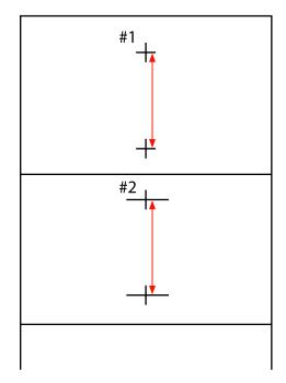
Pattern length is displayed in the control panel. Select the values measured in Step 10.
