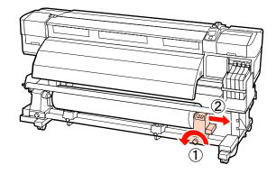
9 Lower the roll onto the roll support.
