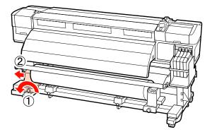
6 Lower the roll onto the roll support.
