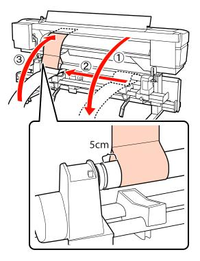
At the front side of the printer, keep the adjustment paper taut and check the positions of the white line on the platen and the line drawn in Step 10.
