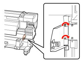
Use the hexagon wrench (large) to tighten and firmly secure the 2 screws.
