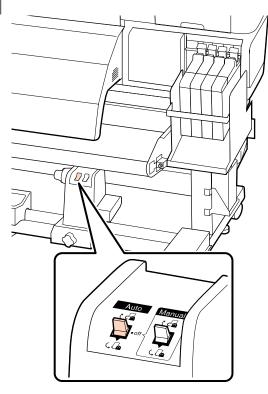
After confirming that the media is loaded correctly, press the ▼ button to feed the media as far as the Auto Take-up Reel Unit roll core holder.
