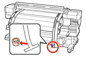
Pull film a from the rear of the printer. Next, loosen the right roll holder fixing screw, and move away the roll holder.
