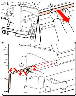
Use a hexagon wrench (large) to rotate the two screws a couple of turns to loosen them.
