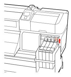
Insert a finger into the depression on the top of the slider and pull straight outward.
