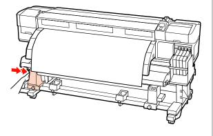
Tighten the left roll core holder locking screw to fix the roll core holder in place.
