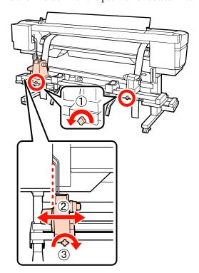
Adjust the right roll holder so that the distance between the two is wider than the roll core.
