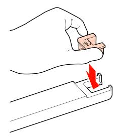
Hold the slider level and insert it, then lower the lock lever.
