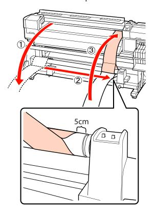
Keep the adjustment paper taut and check the positions of the white line on the platen and the line drawn in Step 6.
