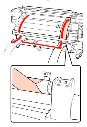
Keep the adjustment paper taut and check the positions of the white line on the platen and the line drawn in Step 6.
