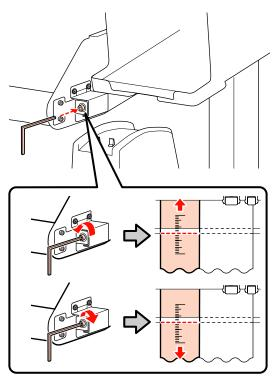
Use the small hexagon wrench to tighten the 2 screws.
