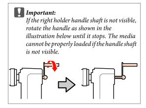
Place media on the roll support oriented according to how it is rolled (see below) and position it as indicated by the mark on the label.
