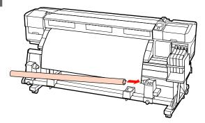
Insert the left holder into the roll core.
