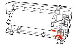
Insert the roll core onto the right holder.
