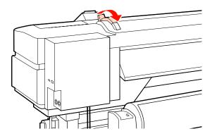
Pull out the media and insert it into the printer.
