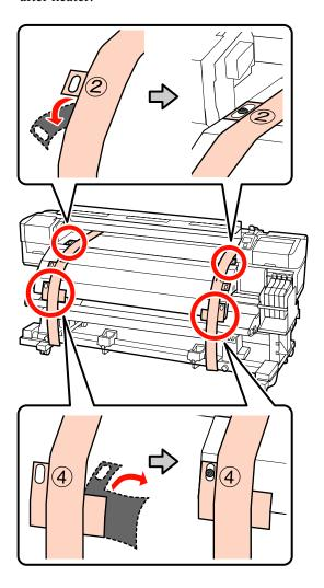
On the rear of the printer, loosen the roll holder fixing screws on the left and right sides. Next, tighten the roll holder fixing screw to align the left roll holder with the position of dotted line.
