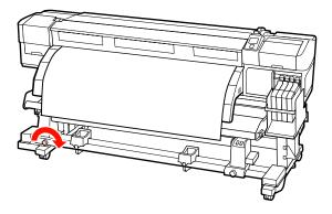
Rotate the handle until part A in the illustration below is fully inserted.
