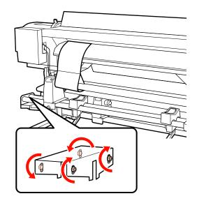
Pull out the adjustment paper from the printer, loosen the right roll holder fixing screw, and move away the roll holder.
