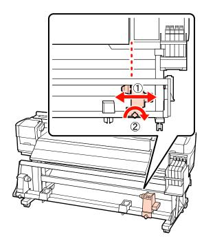
Insert the roll core into the right roll holder.
