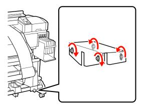
Pull out the adjustment paper from the printer, loosen the left roll core holder locking screw, and remove the roll core holder.
