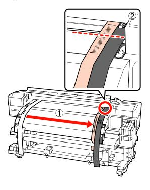
While checking the scale of film a on the front side of the printer, use the large hexagon wrench for adjustment.
