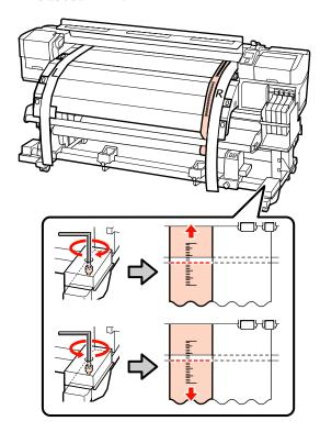
Use the large hexagon wrench to firmly secure the 4 screws.
