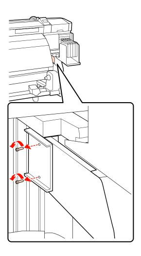
Use a hexagon wrench (large) to rotate the two screws a couple of turns to loosen them.
