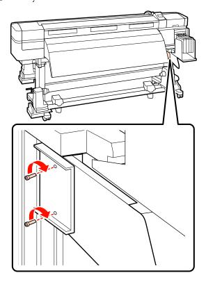
4 Use the hexagon wrench (large) to tighten and firmly secure a screw.
