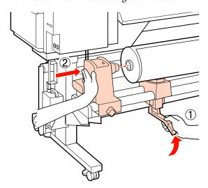
Tighten the roll holder fixing screw until the screw no longer turns to fix the roll holder in place.
