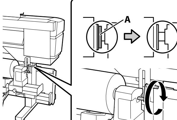
Turn the handle until part A in the upper left figure is hidden. Once part A is hidden, do not turn the handle any further.
