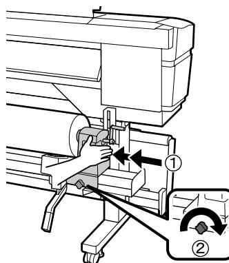
Push the center section on the side of the roll holder towards the roll end twice.
