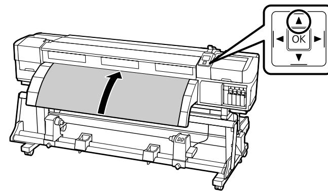
If the media is loaded printable side in, press the ▼ button to rewind the media. We recommend that you press the ► button in the control panel and set **Media Suction** to 2.
