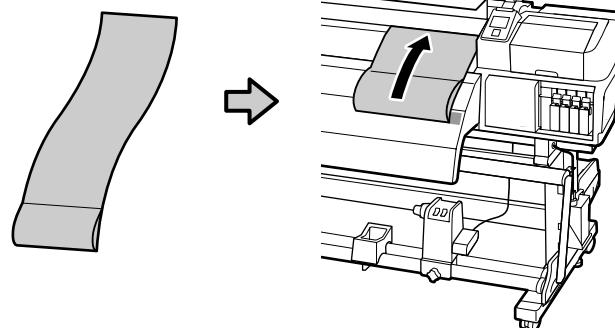
Position the rolled side of the adjustment paper at the bottom, and insert it into the printer from the top end.
