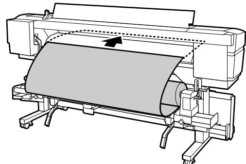
If the left end of the media is not at the center of the rectangular area as shown in the figure on the right, return to step [4].
