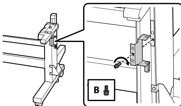
Temporarily fasten the screw as shown in the figure.
