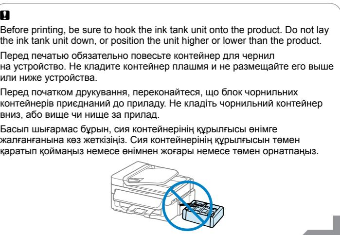
Before printing, be sure to hook the ink tank unit onto the product. Do not lay the ink tank unit down, or position the unit higher or lower than the product.
