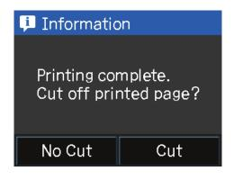
**Cut**: Feeds roll paper to the cutting position.
