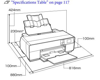
\* When printing on poster board, leave a space of at least 320 mm in behind the printer.
