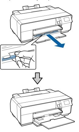
10 With the paper loaded and the printer idle, push the center of the front manual feed tray to close the tray.
