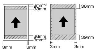
1 Borderless printing is not supported with poster board. 2 Poster board under A3+ in size is printed with 20 mm margins.
