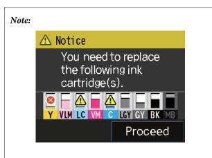
During printing, ink replacement, or when an ink cartridge error has occurred, the level and status of the ink remaining is displayed.
