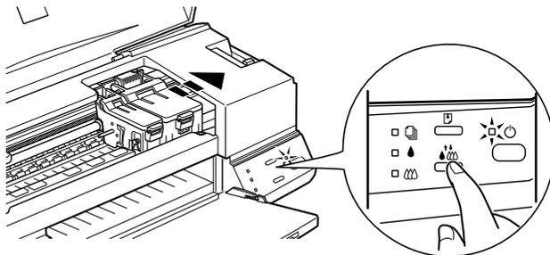
The printer starts cleaning the print head and the
