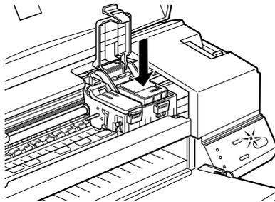
8. Press the ink cartridge clamp down until it locks in place.
