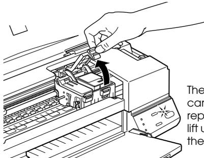
The illustration shows color ink cartridge replacement. To replace the black ink cartridge, lift up only the smaller clamp on the left.
