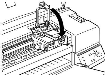
The illustration shows color ink cartridge replacement. To replace the black ink cartridge, lift up only the smaller clamp on the left.
