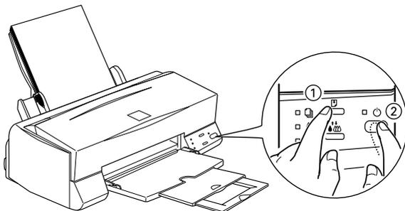
The printer prints an operation check page including your printer's ROM version information, the ink counter code, and a nozzle check pattern. Here are sample printouts.
