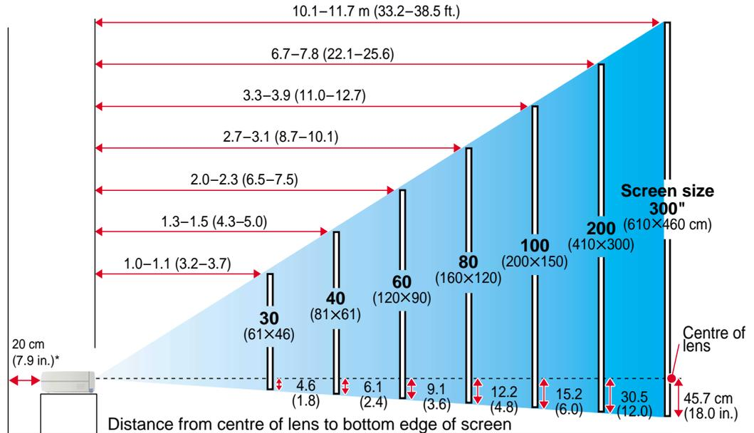
\* When installing against a wall, leave a space of about 20cm (7.9 in.) between the projector and the wall.
