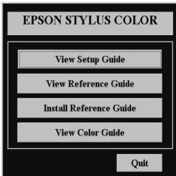
To install the Reference Guide on your hard disk, click Install Reference Guide and follow the on-screen instructions. When installation is complete, a Reference Guide icon appears in the EPSON folder. Double-click the icon to open the guide.
