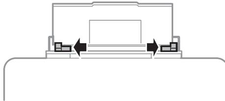
3. Load paper at the center of the rear paper feed with the printable side facing up.
