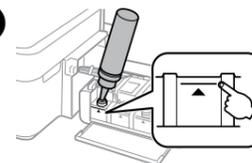
Refer to steps 2 to 9 in section 3 of the front page to refill the tanks to the upper line.
