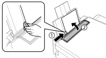
Slide the edge guide against the paper, then close the feeder guard.
