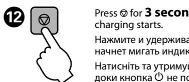
Press for 3 seconds until starts flashing. Ink charging starts.
