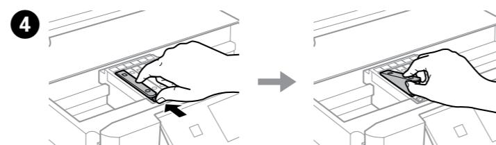
Push the tab to unlock the ink cartridge holder and then remove the cartridge diagonally.
