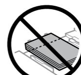
Load paper toward the edge guide with printable side face-down, and check that the paper is not sticking out from the end of the cassette.
