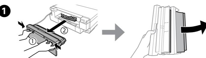
Pull out the rear cover and carefully remove the jammed paper.
