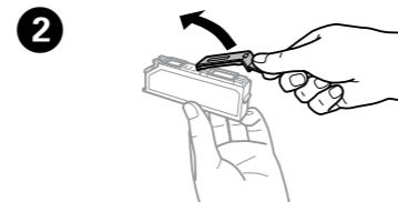
Remove the cap from the new cartridge.
