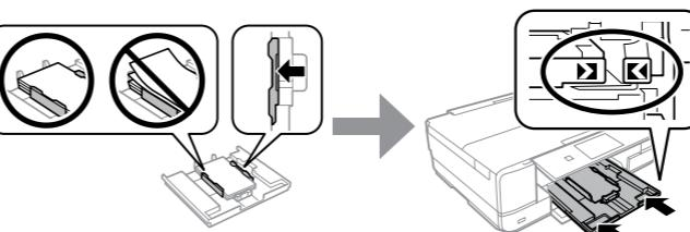
Slide the edge guides to the edges of the paper. Keep the cassette flat and insert it back into the printer carefully and slowly.
