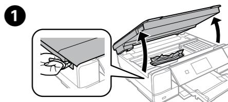
Open the scanner unit and remove all of the paper inside, including any torn pieces.
