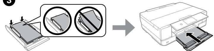
Align the edges of the paper. Keep the cassette flat and insert it back into the printer carefully and slowly.
