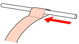
Insert the roll core into the left roll holder. Insert the right roll holder into the roll core, and then tighten the roll holder fixing screw.
