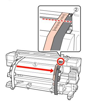
While checking the scale of film a on the front side of the printer, use the large hexagon wrench for adjustment.
