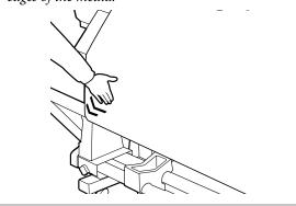
Press the **▼** button to feed the media until the take up roll core begins to turn.
