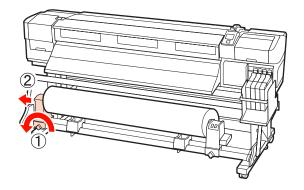
Lower the roll onto the roll support.
