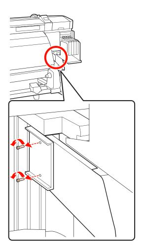
(3) Use a hexagon wrench (large) to rotate the two screws a couple of turns to loosen them.
