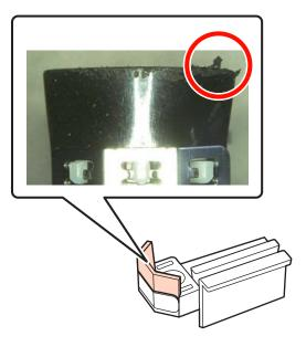
Clean the bottom of the wiper with the cleaning stick (wide).
