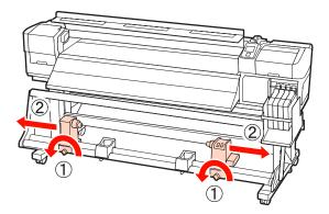
Tighten the roll core holder locking screw to align the right roll core holder with the position of dotted line.
