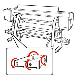
At the front of the printer, remove the counterweight attached to film a.
