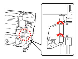
(4) Slide the fixture to the left, and then pull it forward.
