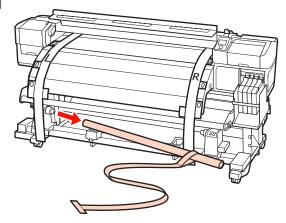
Remove film a from the roll core.
