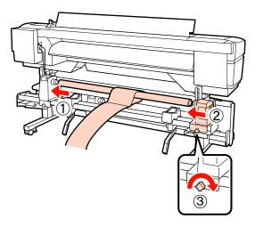
Rotate the handle until part A in the illustration below is fully inserted.
