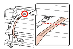
At the front and rear of the printer, raise film a and move it so that it aligns with the right side of film b tightly. After film a stops swinging, check the scale where the front side of the white line of the platen passes.
