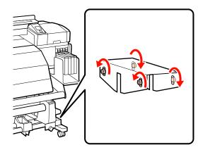
Loosen the roll core holder locking screws and move the left roll core holders to the outside.
