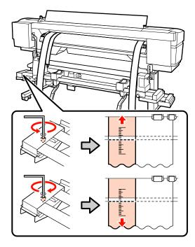
Use the large hexagon wrench to firmly secure the 4 screws.
