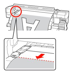
When the Auto Take-up Reel Unit is used on the SC-F7000 Series, raise the tensioner.
