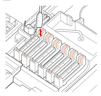
Hold a new cleaning stick in a perpendicular orientation, and wipe off any ink cleaner that has adhered to the inside of the Anti-drying caps.
