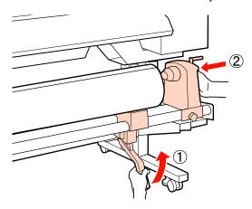
To ensure the roll holder is inserted into the roll core sufficiently, push the center section on the side of the roll holder towards the roll end twice.
