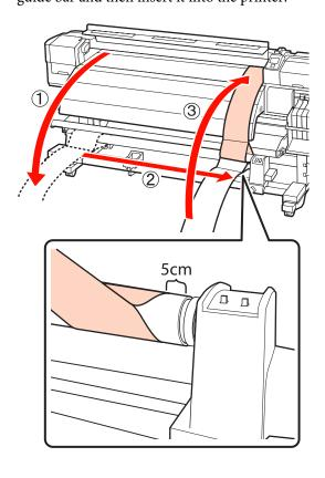
Keep the adjustment paper taut and check the positions of the white line on the platen and the line drawn in Step 13.
