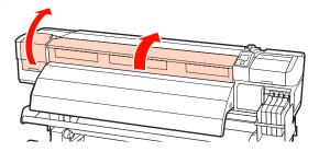
Remove the target media holding plate.
