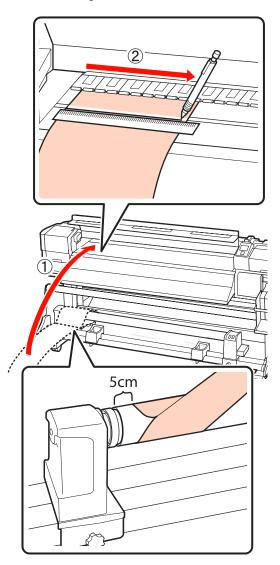
Pull out the adjustment paper, move it to a position 5 cm from the right edge of the roll core, and then insert it into the printer.
