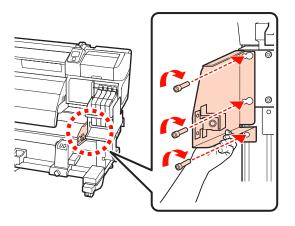
(2) Use the hexagon wrench (small) to tighten and firmly secure the two screws.
