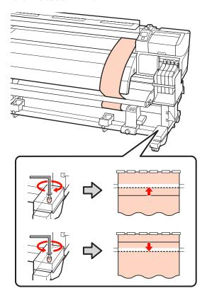
Use the hexagon wrench (large) to tighten and firmly secure the 4 screws.
