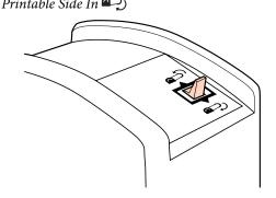
Insert the media past the pressure rollers and lower the media loading lever to hold it in place.
