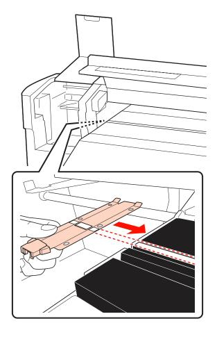
(2) While pressing the tip of the metallic plate against the platen, attach the hooked sections to the front corner of the platen.
