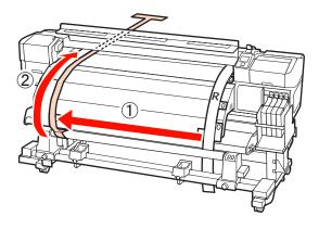
At the front and rear of the printer, raise film a and move it so that it aligns with film b tightly. At the rear of the printer, attach a counterweight to film a.
