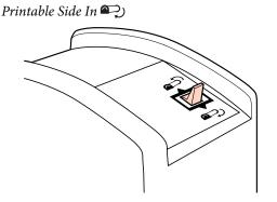
Insert the media past the pressure rollers and lower the media loading lever to hold it in place.
