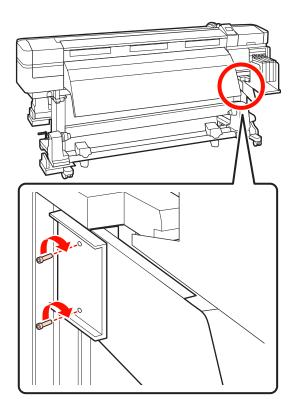
(4) Use the hexagon wrench (large) to tighten and firmly secure a screw.
