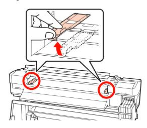
Loosen the roll holder fixing screws sufficiently and adjust the roll holders so that the distance between the two is wider than the media.
