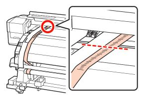
At the front and rear of the printer, raise film a and move it so that it aligns with the right side of film b tightly. After film a stops swinging, check the scale where the front side of the white line of the platen passes.
