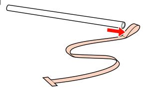
Remove the left and right side of film b from the printer.
