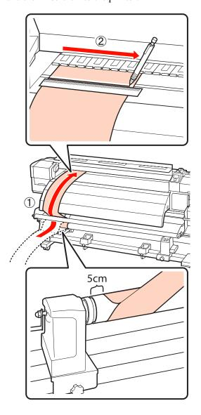
Pull out the adjustment paper, move it to a position 5 cm from the right edge of the roll core, and then insert it into the printer.
