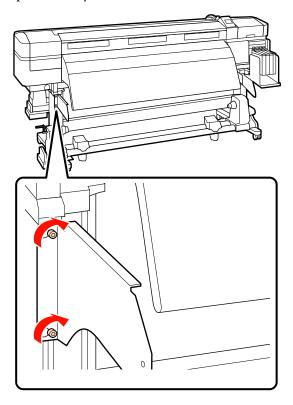
Use the hexagon wrench (small) to tighten the four screws and secure the media guide bar.
