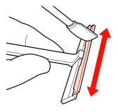
Wipe away ink stains and so on from the print head surface by moving the cleaning wiper from the inside toward you once.
