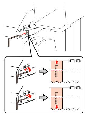
Use the small hexagon wrench to tighten the 2 screws.
