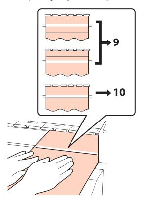
While checking the state of the two lines on the front side of the printer, use the hexagon wrench (large) to adjust the screw so that the drawn line aligns with the position of the dotted line.
