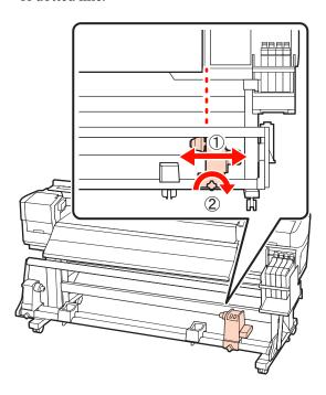
Insert the roll core into the right roll holder.
