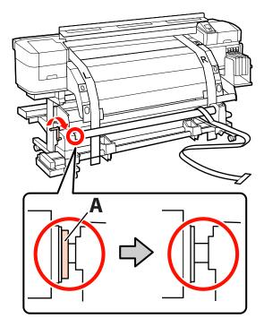
Bring film a to the left side of film b. Pass the lead edge of film a between the media guide bar and after heater, and then insert it into the printer.
