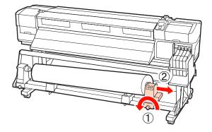
Lower the roll onto the roll support.
