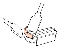
If the wiper part has split off or is broken, we recommend replacing it with a new one.
