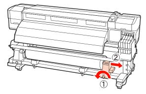
Lower the roll onto the roll support.
