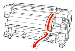
Bring the adjustment paper to a position 5 cm from the left edge of the roll core. Pass the lead edge of the adjustment paper by the front of the media guide bar and then insert it into the printer.
