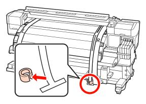
Pull film a from the rear of the printer. Next, loosen the right roll holder fixing screw, and move away the roll holder.
