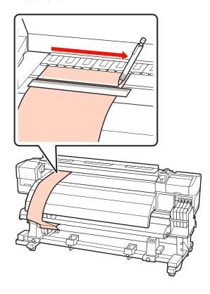
Pull out the adjustment paper. Bring the adjustment paper to a position 5 cm from the right edge of the roll core. Pass the lead edge of the adjustment paper by the front of the media guide bar and then insert it into the printer.
