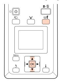
Pressing the 🗗 button when the printer is ready to print displays the Maintenance menu.
