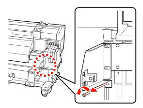
(2) Use a hexagon wrench (large) to remove two screws.
