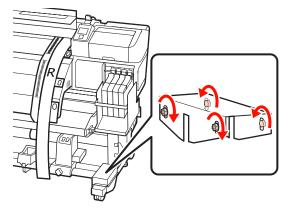
At the rear of the printer, remove the counterweight attached to film a.
