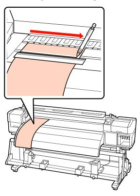
Pull out the adjustment paper from the rear side, move it to a position 5 cm from the left edge of the roll core, and then insert it into the printer.
