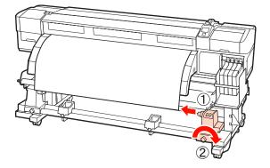
5 Insert the roll core onto the right holder.
