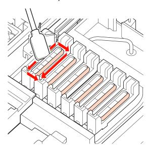
Wipe off ink that has adhered to the guide section.
