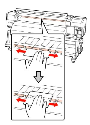
Wipe lint, dust, and adhered ink from the platen using a brush or soft cloth that has been soaked in water and squeezed well.
