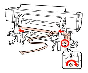
Rotate the handle until part A in the illustration below is fully inserted.
