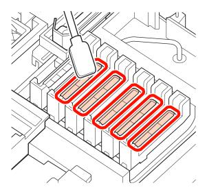
Hold the cleaning stick (narrow) in a perpendicular orientation, and wipe the outer areas of all the caps.
