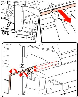
Use a hexagon wrench (large) to rotate the two screws a couple of turns to loosen them.
