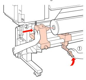
Tighten the roll holder fixing screw until the screw no longer turns to fix the roll holder in place.
