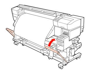
Open the front cover, and move the media holding plates out of the way.
