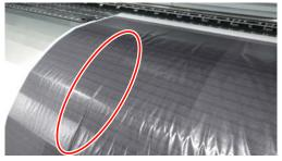
If thin media or media lengthened by water absorption is printed at a high density is being taken up, creases may appear in the media in the after heater. In the setup menu, set **Take-up Tension** to **Manual**, and set the value to **Lv1** or **Lv2**. Alternatively, we recommend using thicker media.
