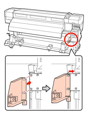
(2) Use the hexagon wrench (large) to tighten and firmly secure the two screws that were provisionally secured.
