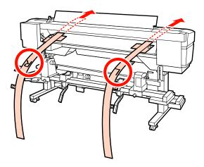
As shown in the illustration, align Hole 1 of film b with the screws on the left and right edges of the loading guide, and then adhere it.
