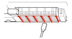
Dampen the cleaning stick (wide) with the ink cleaner, then wipe away any dust and dirt on the front, back, and sides of the wiper blade.
