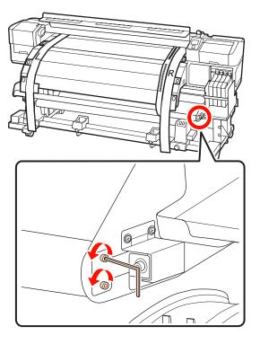
While checking the scale of film a on the front side of the printer, make adjustments using the large hexagon wrench while you use your hand to hold the media guide bar.
