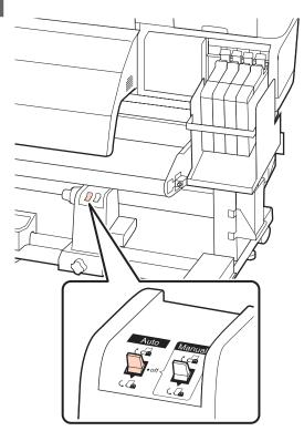
After confirming that the media is loaded correctly, press the ▼ button to feed the media as far as the Auto Take-up Reel Unit roll core holder.
