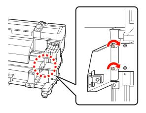
(3) Use the hexagon wrench (large) to tighten and firmly secure the 2 screws.
