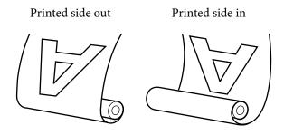
Taking-up with printed side out places the printed surface on the outside of the roll.
