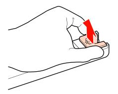
Attach the chip unit supplied with the new ink pack to the slider.
