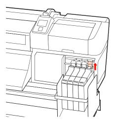
Insert a finger into the depression on the top of the slider and pull straight outward.
