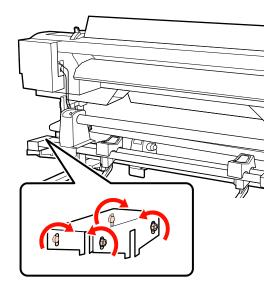
Pass the left and right sides of film b from the rear to the front.
