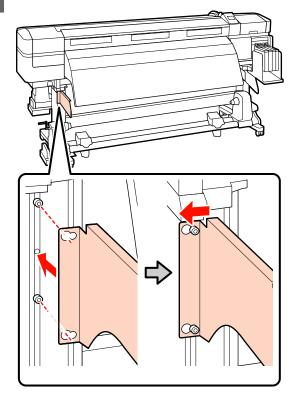
Use the hexagon wrench (large) to tighten and firmly secure the two screws that were provisionally secured.
