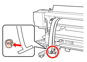
Pull out film a from the printer. Next, loosen the right roll core holder locking screw and remove the roll core holder from the roll.
