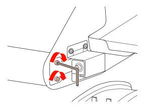
At the rear of the printer, remove the counterweight attached to film a.
