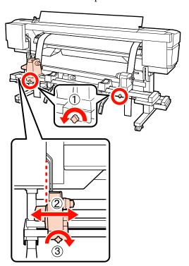
Adjust the right roll holder so that the distance between the two is wider than the roll core.
