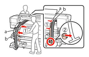
After film a stops swinging, record the value of the scale on the front side of the white line of the platen.
