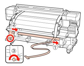
Rotate the handle until part A in the illustration below is fully inserted.
