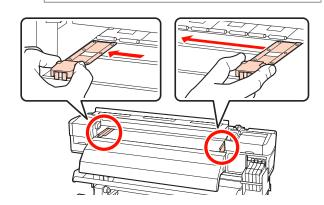
(2) Remove the left media holding plate, and then remove the right one.
