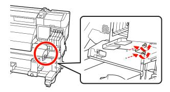
(2) While supporting the fixture, use a hexagon wrench (large) to remove the three screws.
