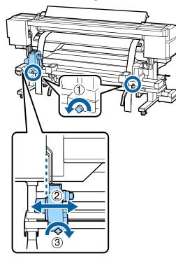
Adjust the right roll holder so that the distance between the two is wider than the roll core.
