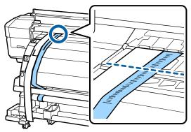
At the front and rear of the printer, raise film a and move it so that it aligns with the right side of film b tightly. After film a stops swinging, check the scale at the edge of the plate on the platen and on film a.
