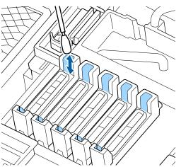
Hold a new cleaning stick in a perpendicular orientation, and wipe off any ink cleaner that has adhered to the inside of the Anti-drying caps.
