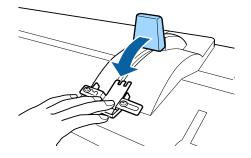
When you lower the media loading lever, the media confirmation and setting changes are displayed on the control panel screen. See the following and check the settings.
