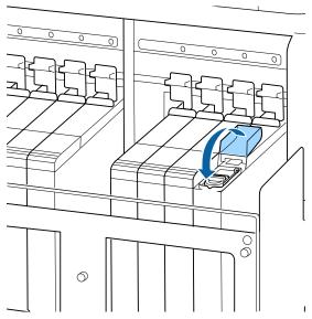
When ink adheres to the heat shield when refilling the ink, remove the heat shield and clean it.
