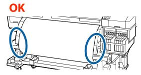
If the tensions of the left and right edges of the media are different, the media cannot be taken up correctly. Return to step 1.
