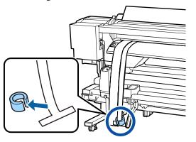
21 Pull out film a from the printer. Next, loosen the right roll core holder locking screw and remove the roll core holder from the roll.
