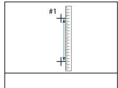
When the Feed Speed is set to Lv2 #1 and #2 are printed. Check both patterns.
