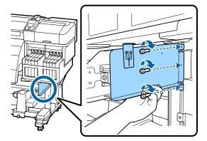
Secure the tank cover adjustment section.
