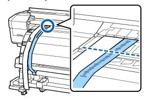
16 At the front and rear of the printer, raise film a and move it so that it aligns with the right side of film b tightly. After film a stops swinging, check the scale at the edge of the plate on the platen and on film a.
