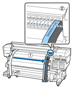
While checking the scale of film a at the front of the printer, make an adjustment on the rear side
