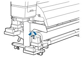
To prevent the media from sliding off the roll, support the roll at its left end.
