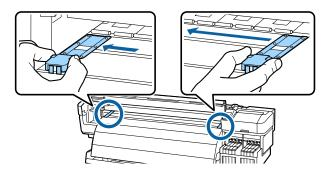
(2) Remove the left media holding plate, and then remove the right one.
