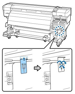
Attach the left-hand fixing plate for the media guide bar.
