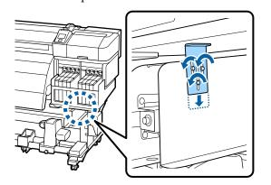
Remove the tank cover holding plate.
