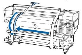
While checking at the front and rear of the printer, align film a with film b tightly. At the rear of the printer, attach a counterweight to film a.
