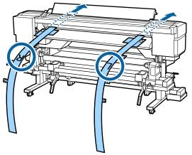
5 As shown in the illustration, align Hole 1 of film b with the screws on the left and right edges of the loading guide, and then adhere it.
