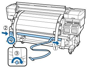
**4** Rotate the handle until part A in the illustration below is fully inserted.
