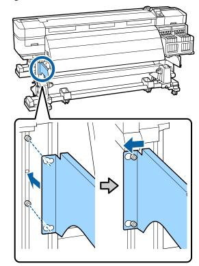
6 Use the hexagon wrench (large) to tighten and firmly secure the two screws that were provisionally secured.
