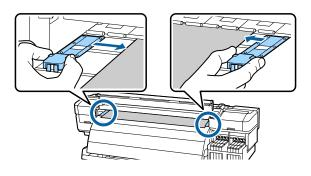
(2) Adjust so that the edge of the media is aligned to the center of the round holes in the media holding plates.
