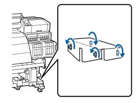
2 Loosen the roll core holder locking screws and move the left roll core holders to the outside. Next, tighten the roll core holder locking screw to align the right roll core holder with the position of dotted line.
