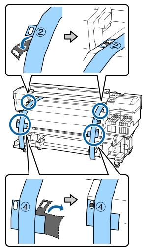
7 On the rear of the printer, loosen the roll holder fixing screws on the left and right sides. Next, tighten the roll holder fixing screw to align the left roll holder with the position of dotted line.
