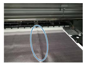
When using thin media or media lengthened by water absorption, vertical creases may occur between the pressure rollers. When vertical creases occur in media on the platen, head striking may occur. Perform the following sequence until the vertical creases have improved.
