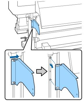
5 Loosen the tank cover adjustment section. Use a hexagon wrench (small) to rotate the three screws a couple of turns to loosen them.
