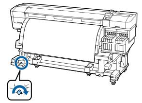
Rotate the handle until part A in the illustration below is fully inserted.
