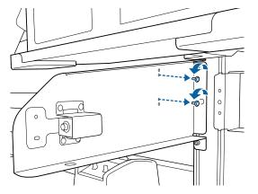
8 Remove the right-hand fixing plate for the media guide bar.
