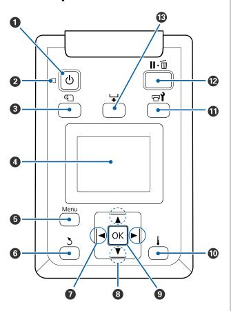
• U button (power button) Turns the power on and off.
