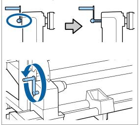
Insert the roll core into the right roll holder. Next, insert the left roll core holder into the roll core, and then tighten the roll core holder locking screw.
