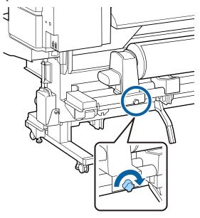
Raise the lift lever on the right side of the printer to lift the media into position, then firmly insert the roll holder.
