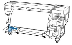
8 Tighten the left roll core holder locking screw to fix the roll core holder in place.
