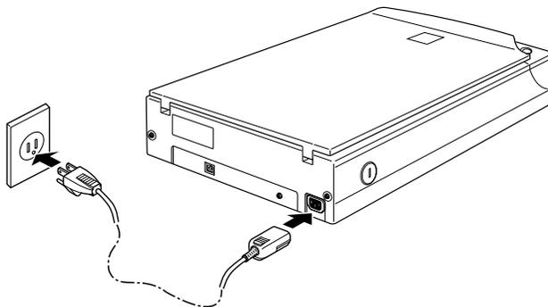
If the power cord is not attached to the scanner, connect it to the AC inlet on the back of the scanner, and plug the other end into a properly grounded electrical outlet.
