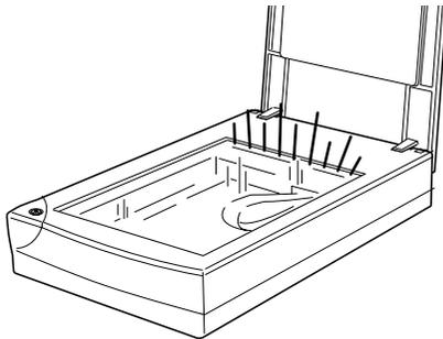
5. The fluorescent lamp stays on, meaning the scanner has completed initialization.
