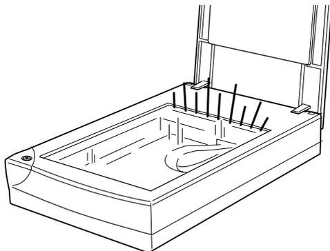
2. Turn on the computer and make sure that the scanner's fluorescent lamp is on, and not flashing.
