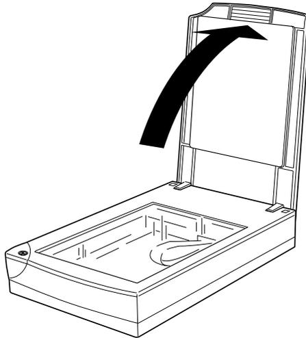
4. Place the document on the document table, with the side to be scanned facing down. Make sure that the document is carefully aligned.
