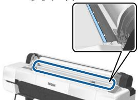
□ For Epson Color Calibration Utility color charts, insert the page from the top with the printed side facing up.
