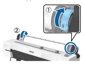
After removing the paper, reload the paper and restart printing.
