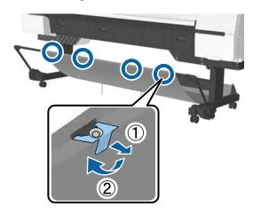
2 Loosely roll up the removed cloth with the top surface of the cloth inside, and insert the loop into the clamps hanging down from the printer.
