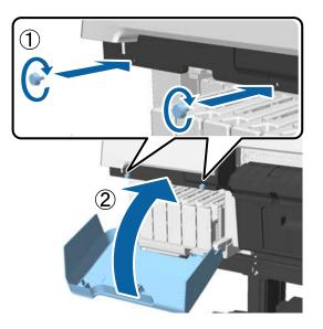
Open the printer cover, and then use a cleaning stick to wipe away dirt on the top edges of the cap (two points).
