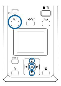
Press the  $\mathbb{T}$  button on the control panel. Use the  $\mathbf{\nabla}/\mathbf{\Delta}$  buttons to select **Use Take-up Unit**, and then press the **OK** button.
