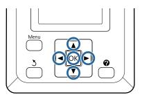
Press the **◄**/**▶** buttons on the control panel to highlight **●** and press the OK button.
