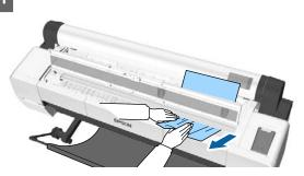
After removing the paper, reload the paper and restart printing.
