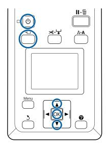
1 Turn on the printer by pressing the  $\bigcirc$  button.
