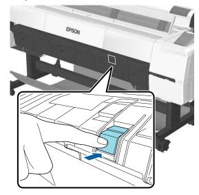
*Press the back side of the part, as shown below, to return the part to its original position.*
