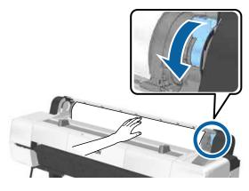
When **Auto Loading** is set to **Off**, you can cut the edge of the roll paper with the built-in cutter by pressing the **OK** button, and then pressing the  $\prec \cdot \downarrow$  button within 5 seconds.
