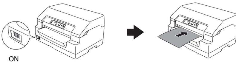
Insert a single sheet printable side up into the front slot until the top part of the paper reaches the roller inside. The printer loads the paper automatically to the correct position and the paper is ready to be printed.
