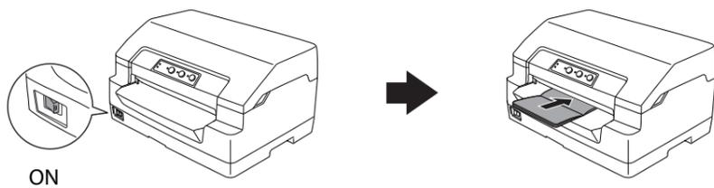
Open your passbook to the page to be printed. Then insert the passbook printable side up and the magnetic tape facing away from the printer into the front slot until the top part of it reaches the roller inside. The printer loads it automatically to the correct position and the passbook is ready to be printed.
