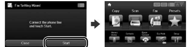
When the fax setting wizard screen is displayed, tap start to configure the minimum settings for fax features. If you do not want to configure them now, close the fax setting screen. The home screen is displayed and printer is ready for printing.
