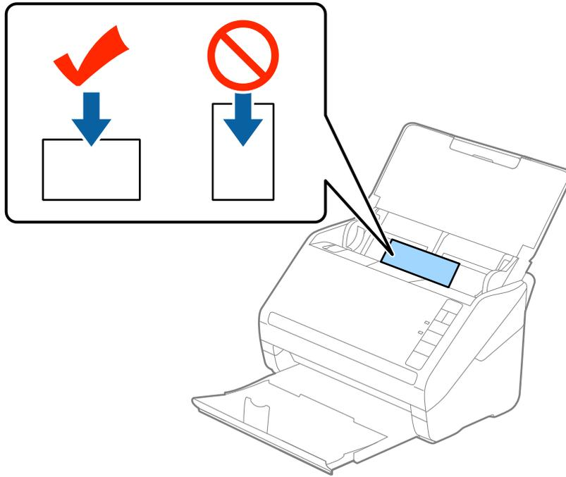
4. Slide the edge guides to fit the edge of the plastic cards.
