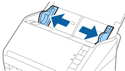
3. Load the laminated cards into the input tray facing down with the top edge facing into the ADF. Slide the laminated cards into the ADF until they meet resistance.
