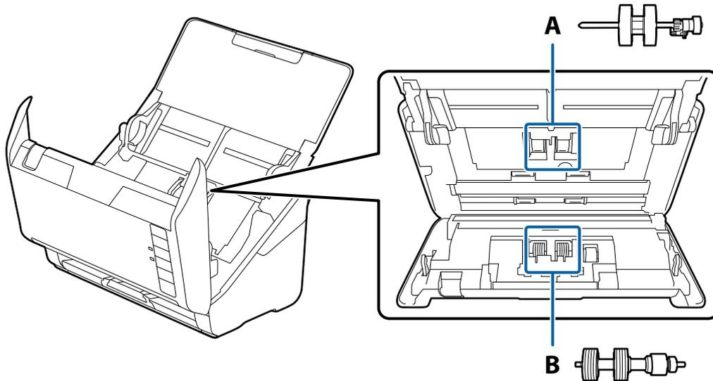
A: pickup roller, B: separation roller
