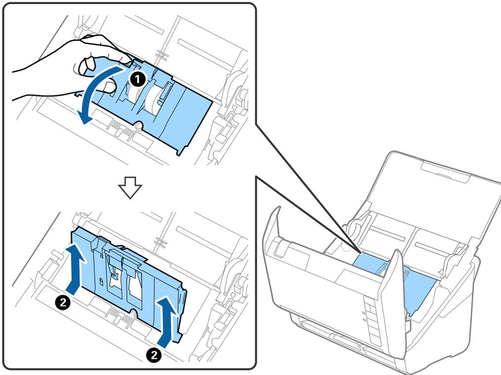
5. Pull down the fixture of the roller axis, and then slide and remove the installed pickup rollers.
