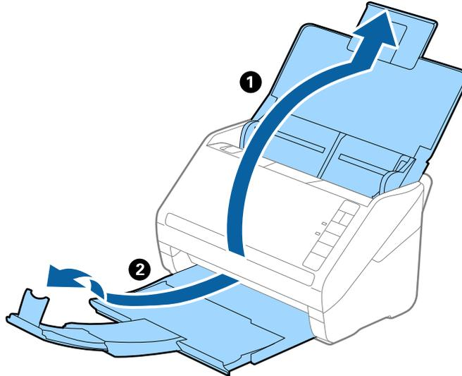
2. Slide the edge guides on the input tray all the way out.
