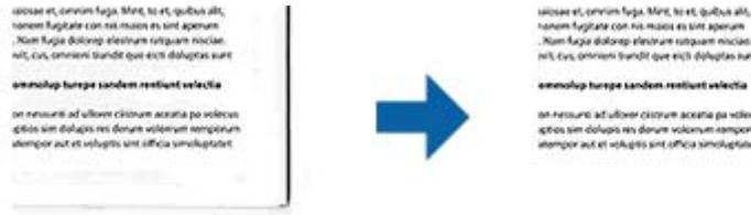
For double-sided scanning, the settings for the edge fill range are mirror-reversed for the back of the original.
