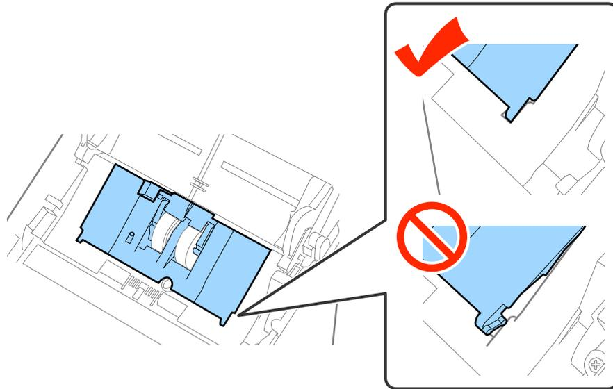
8. Push the hooks on both ends of the separation roller cover to open the cover.
