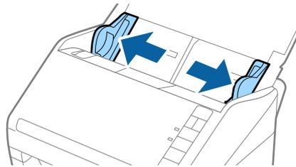
3. Place the Carrier Sheet with the illustration on the front edge facing up and place the photo in the center of the Carrier Sheet with the side to be scanned facing down.
