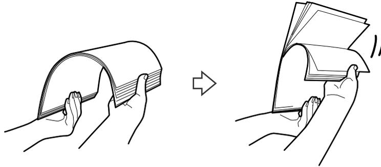
4. Align the edges of the originals with the printed side facing down and slide the leading edge into a wedge shape.
