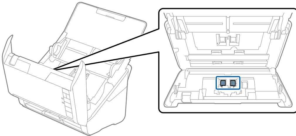
7. Wipe off any stains on the separation roller using a soft cloth or a genuine Epson cleaning kit.
