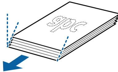
5. Load the originals into the input tray facing down with the top edge facing into the ADF.
