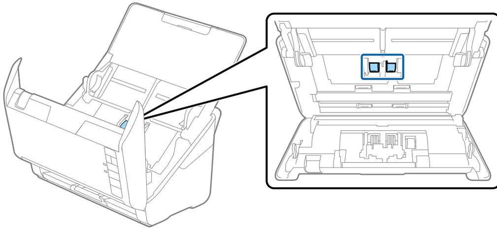
9. Wipe off any stains on the pickup roller using a soft cloth or a genuine Epson cleaning kit.
