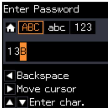
5. Press the ► button once to move the cursor, and then press the ⬆ button to switch the character type to abc. Press the ▼ button twice to select "y".
