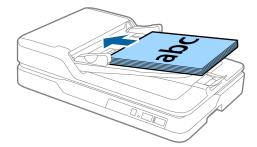
4. Slide the edge guides to fit the edge of the originals making sure there are no gaps between the originals and the edge guides. Otherwise, the originals may be fed askew.
