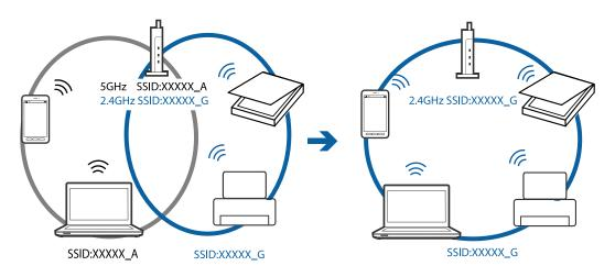
□ Most access points have a privacy separator feature that blocks communication between connected devices. If you cannot communicate between the scanner and the computer or smart device even if they are connected to the same network, disable the privacy separator on the access point. See the manual provided with the access point for details.
