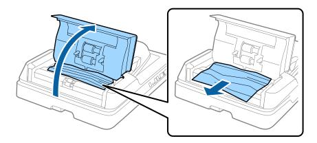
3. If you cannot remove the originals, raise the ADF. Make sure the ADF cover is open while you raise the ADF.
