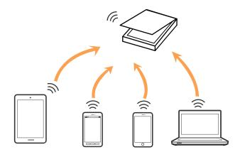
The scanner can be connected by Wi-Fi and AP mode simultaneously. However, if you start a network connection in AP mode when the scanner is connected by Wi-Fi, the Wi-Fi is temporarily disconnected.
