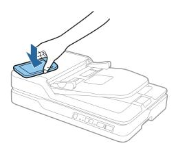
3. Touch the NFC antenna of your smart device to the scanner's NFC tag.
