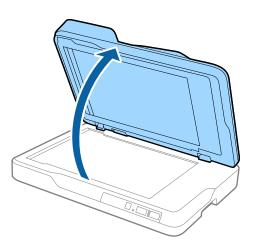
2. Place your original face down on the scanner glass making sure the upper corner of the side you want to scan is against the corner of the scanner next to the arrow mark.
