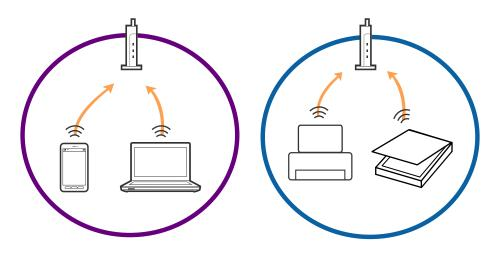
You may not be able to connect to the access point when the access point has multiple SSIDs and devices are connected to different SSIDs on the same access point. Connect the computer or smart device to the same SSID as the scanner.
