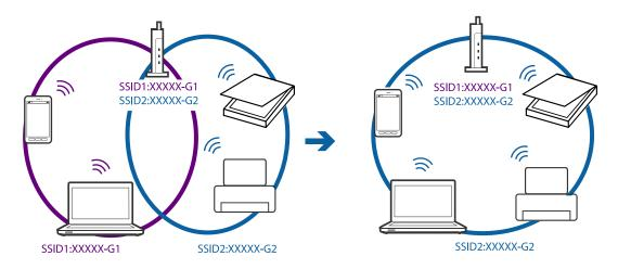
□ An access point that is compliant with both IEEE802.11a and IEEE802.11g has SSIDs of 2.4 GHz and 5 GHz. If you connect the computer or smart device to a 5 GHz SSID, you cannot connect to the scanner because the scanner only supports communication over 2.4 GHz. Connect the computer or smart device to the same SSID as the scanner.
