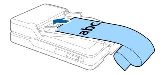
3. Adjust the edge guides to fit the edge of the long paper making sure there is no gap between the paper edge and the edge guide. Otherwise, the originals may be fed askew or jammed.
