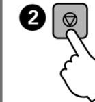
Run print head cleaning until all lines are printed completely. Hold down  $\text{Ⓢ}$  for 3 seconds until the power light starts flashing. Print head cleaning starts.
