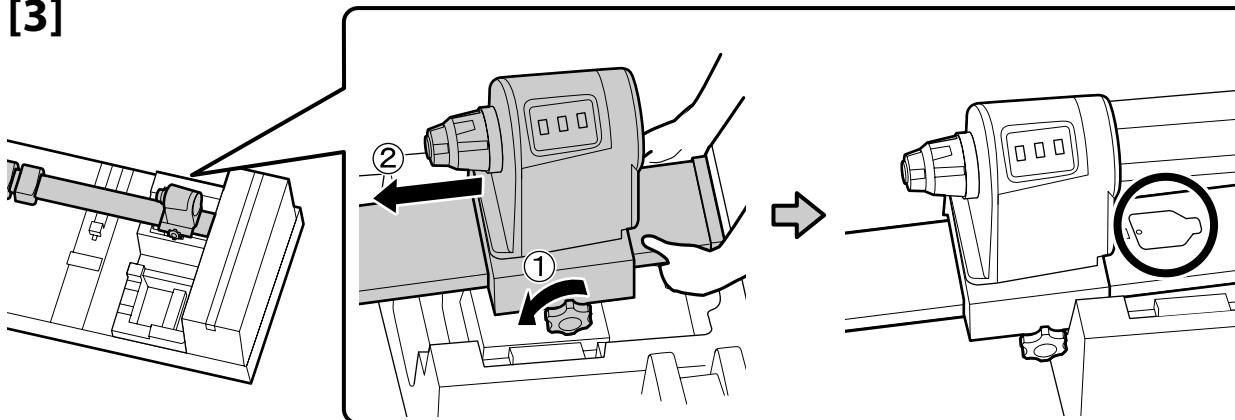
Lift the end, loosen the lock screw, and move the unit into position.
