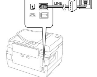
RJ-11 Phone Line / RJ-11 Telephone set connection
