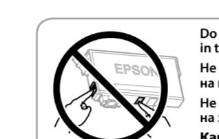
Do not touch the sections shown in the illustration of the cartridge.
