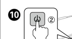
Turn on the printer and wait until it stops flashing.
