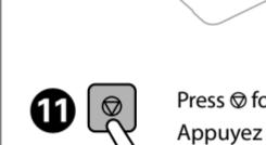
Press the for 3 seconds until it starts flashing. Ink charging starts.
