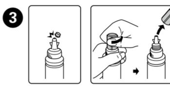
Snap off the top of the cap or remove the cap cover.
