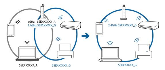
☐ Most access points have a privacy separator feature that blocks communication between connected devices. If you cannot communicate between the printer and the computer or smart device even if they are connected to the same network, disable the privacy separator on the access point. See the manual provided with the access point for details.
