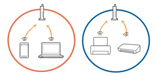
☐ You may not be able to connect to the access point when the access point has multiple SSIDs and devices are connected to different SSIDs on the same access point. Connect the computer or smart device to the same SSID as the printer.
