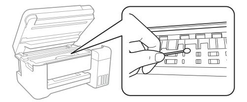
Do not touch the white flat cable, translucent film, and ink tubes inside the printer. Doing so may cause a malfunction.
