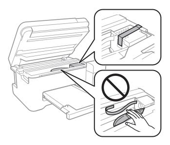
7. Make sure to install the cap onto the ink tank securely.
