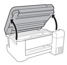
3. Check if the translucent film is smeared. Smears are easier to see if you use a light. If there are smears (such as finger marks or grease) on the translucent film (A), go to the next step.
