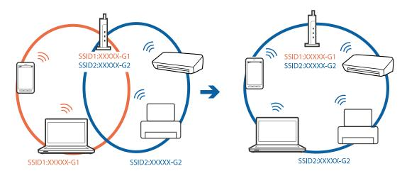
☐ An access point that is compliant with both IEEE802.11a and IEEE802.11g has SSIDs of 2.4 GHz and 5 GHz. If you connect the computer or smart device to a 5 GHz SSID, you cannot connect to the printer because the printer only supports communication over 2.4 GHz. Connect the computer or smart device to the same SSID as the printer.
