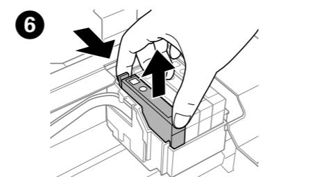
Squeeze the tab on the ink cartridge and lift it out.
