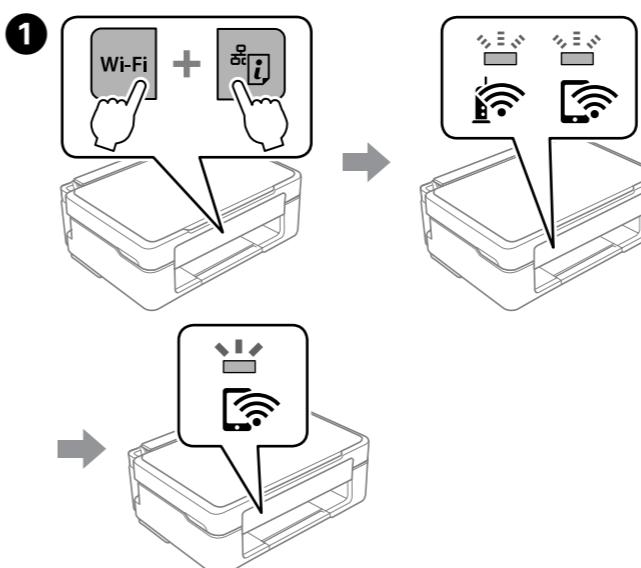
While holding down the , press the button until the light and the light flash alternately. Wait until the process ends. When a connection is established, the light turns on.
