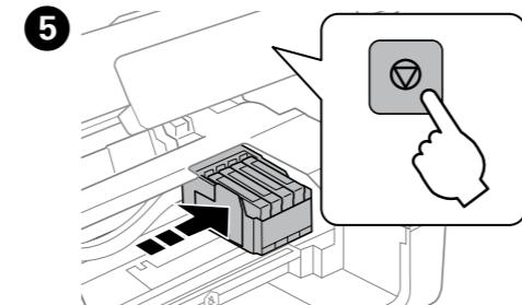
Press again to move the print head to the ink cartridge replacement position.
