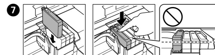
Insert the new ink cartridge and press it down firmly.
