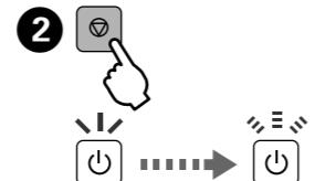
Run the print head cleaning. Hold down
