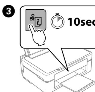
Hold down the button on the printer for at least 10 seconds. The network status sheet is printed. You can check the SSID and Password for Wi-Fi Direct (Simple AP).
