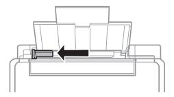
3. Load paper vertically along the right side of the rear paper feed with the printable side facing up.
