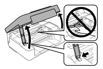
2. Hold down the  $\bigcirc$  button until the ink cartridge holder starts moving.
