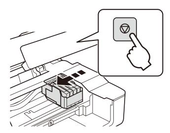
The ink cartridge holder moves to the replacement position.
