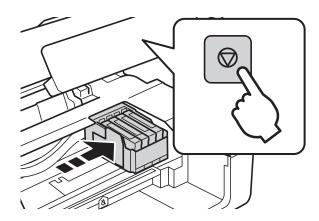
4. When replacing the black ink cartridge, gently shake the new black ink cartridge four or five times and then remove it from its package. When replacing other color cartridges, remove the new color cartridges from their package without shaking.
