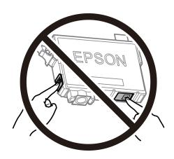
5. Squeeze the tab on the ink cartridge and pull it straight up. If you cannot remove the ink cartridge, pull it firmly
