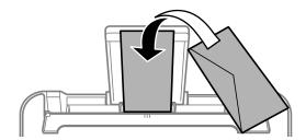
☐ Fan and align the edges of the envelopes before loading. When the stacked envelopes are puffed up with air, press them down to flatten them before loading.
