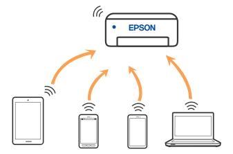
The printer can be connected by Wi-Fi and Wi-Fi Direct (Simple AP) connection simultaneously. However, if you start a network connection in Wi-Fi Direct (Simple AP) connection when the printer is connected by Wi-Fi, the Wi-Fi is temporarily disconnected.
