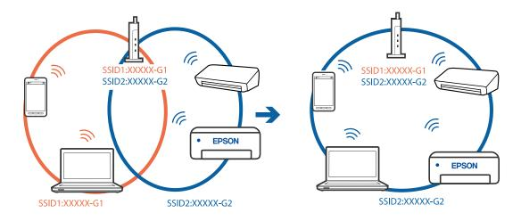
□ A wireless router that is compliant with both IEEE802.11a and IEEE802.11g has SSIDs of 2.4 GHz and 5 GHz. If you connect the computer or smart device to a 5 GHz SSID, you cannot connect to the printer because the printer only supports communication over 2.4 GHz. Connect the computer or smart device to the same SSID as the printer.
