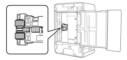
Return the printer to its normal position, and then insert the paper cassette.
