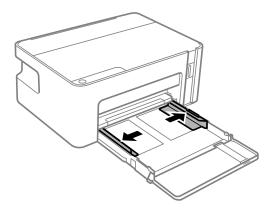
3. With the printable side facing down, load paper until it touches the back of the paper cassette.
