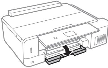
4. Check that the printer is not operating, and then pull out paper cassette 1. Paper cassette 1 has an alignment mark
