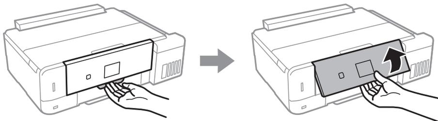
2. When the output tray is ejected, check that there is no paper on the tray, and then close it by pushing it with your hand.
