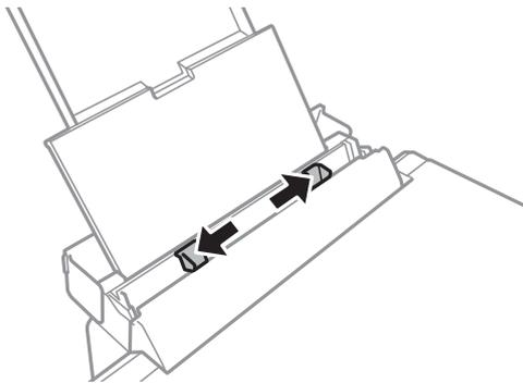
4. Load paper at the center of the rear paper feed with the printable side facing up.
