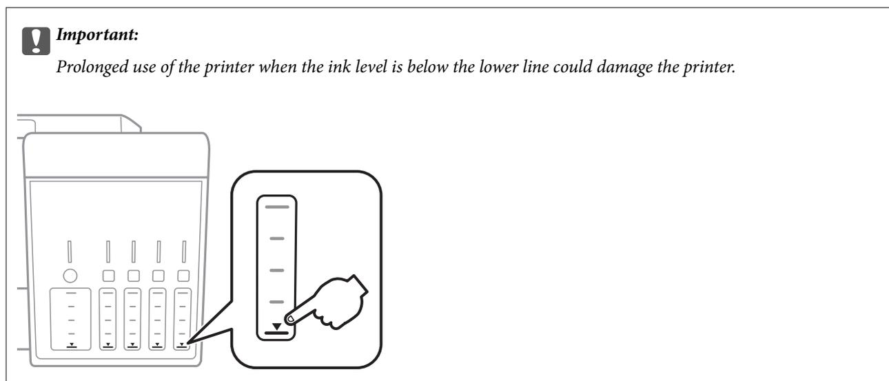
You can check the approximate ink levels from the computer, and the approximate service life of the maintenance box from the control panel or the computer.
