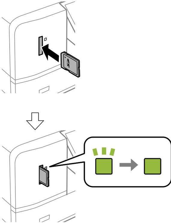
2. When you have finished using the memory card, make sure the light is not flashing, and then remove the card.
