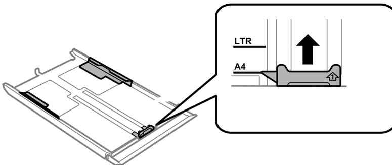
7. With the printable side facing down, load paper against the front edge guide.
