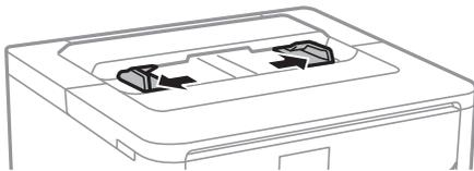
2. Load paper at the center of the paper feed slot with the printable side facing down.
