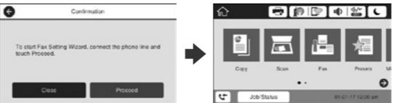
When the fax setting wizard screen is displayed, tap proceed to configure the minimum settings for fax features. If you do not setting now, close the fax setting screen. The home screen is displayed and printer is ready for printing.
