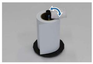
Insert the flange into the shaft of the spindle unit so that the core of the roll paper is held securely between the top and bottom flanges.
