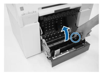
Check that there is no paper, foreign material, or scrap paper at the back of the printer. If there is a jam, remove the paper slowly.
