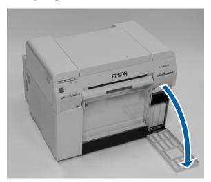
Be careful not to tilt the maintenance cartridge, and remove it carefully.
