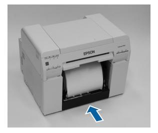
7 Carefully roll the paper into the printer to take up any slack.
