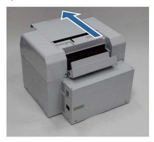
If a lot of paper has been ejected from the front of the printer, cut the paper in front of the jam with a pair of scissors and so on.
