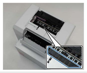
Cut the paper you have pulled out with scissors and so on. Remove the cut section.
