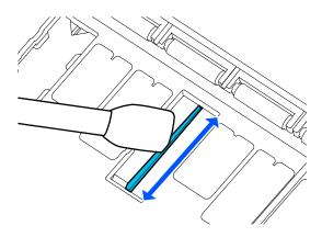
Bend a new pad for borderless printing as shown in the illustration.
