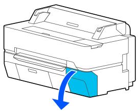
Remove the new ink cartridge from the bag. Shake the ink cartridge for 10 seconds 30 times horizontally in approximately 5 cm movements as shown in the illustration.
