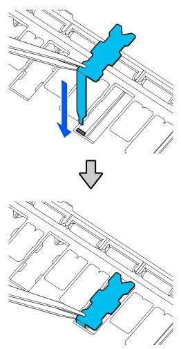
Push the protrusions on the left and right of the pads for borderless printing into the grooves on the left and right.
