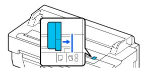
Face the scanning side upward and align the right edge of the document with the document guide. Insert the leading edge of the document into the scanner's paper slot until you hear a beep.
