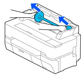
Pull off the transparent flange from the spindle.
