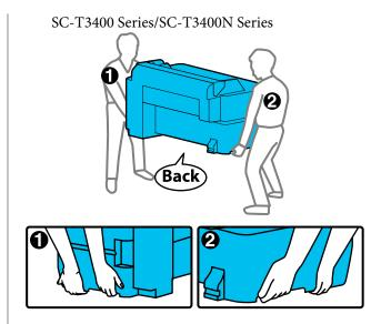
Do not tilt the product more than 10 degrees forward, back, left, or right while moving it. Failure to observe this precaution could result in the printer falling over, causing accidents.
