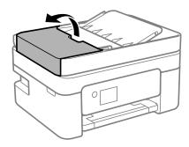
2. Use a soft, moist cloth to clean the roller and the interior of the ADF.
