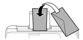
☐ Fan and align the edges of the envelopes before loading. When the stacked envelopes are puffed up with air, press them down to flatten them before loading.
