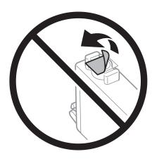
☐ Do not touch the sections shown in the illustration. Doing so may prevent normal operation and printing.
