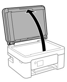
2. Use a soft, dry, clean cloth to clean the surface of the scanner glass.
