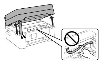
3. Check if the translucent film is smeared. Smears are easier to see if you use a light. If there are smears (such as finger marks or grease) on the translucent film (A), go to the next step.
