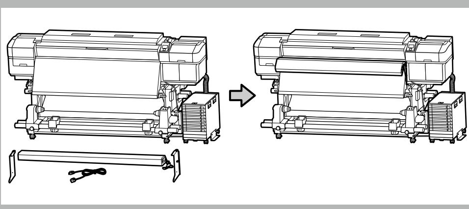
**!** Install the additional print-drying system\* as described in the manual supplied with the system.
