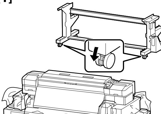
Before using the printer, be sure the stand is fixed in place. When moving the printer unlock the casters.
