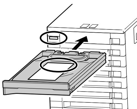
After confirming that the colors of the labels on the ink supply unit and ink unit match, slide the tray in until it contacts the back of the slot.
