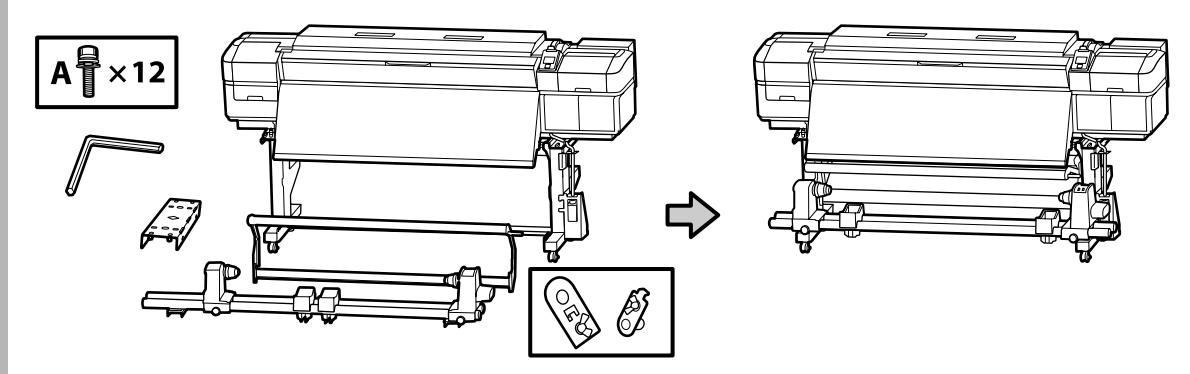
**[1]** Carry the Auto Take-up Reel Unit using two persons, each holding the two bars as shown in the figure on the right.
