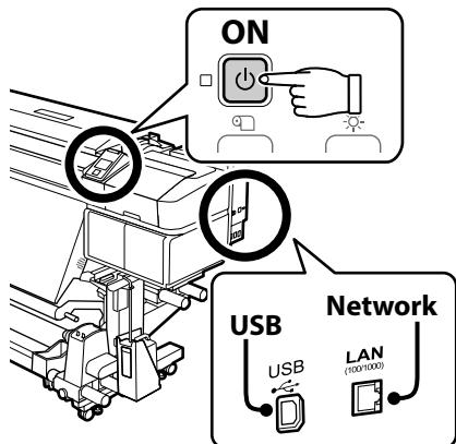
Ready the printer and computer for connection before proceeding, but do not connect the cables until the installer prompts you to do so. The basic software will not be installed if the devices are not connected according to the on-screen instructions.
