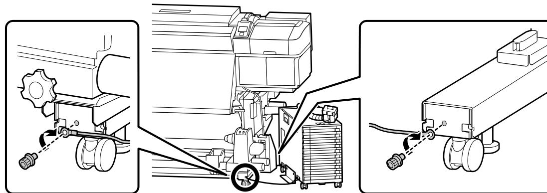
Be sure to secure the restraining wire to front and back of the printer leg using screws. If the ink unit is not secured with the restraining wire, the ink tube may be damaged if the ink unit is moved while the ink unit is connected.
