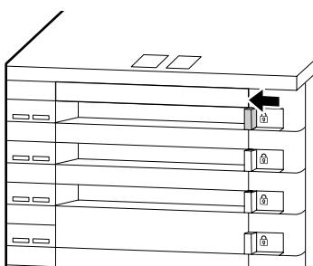
Repeat Steps 1 to 5 to place the ink supply units for the remaining colors in the trays and insert the trays in the ink unit.
