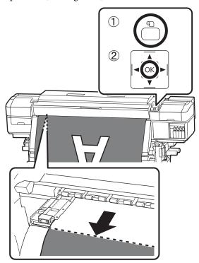
If you have printed the amount of media remaining, press the ▲ button to rewind the media so that this information will remain on the unprinted roll after the media is cut.
