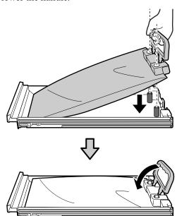
While the ink supply unit is in the tray, as shown in the illustration below, carefully shake it by tilting it up and down at about a 60 degree angle 5 times in 5 seconds.
