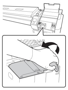
Grip the sides, and pull it straight up to lift it out.
