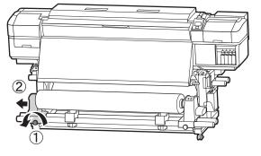
3 Lower the roll onto the roll support.
