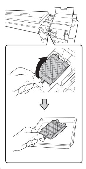
Insert the two hooks on the flushing pad into the slots on the printer and press the tab down until the pad clicks into place.
