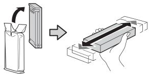
Match the color of the cartridge to the color of the label on the printer and insert.
