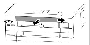
While the ink supply unit is in the tray, as shown in the illustration below, carefully shake it by tilting it up and down at about a 60 degree angle 5 times in 5 seconds.
