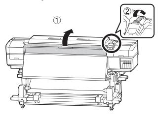
While holding the tabs of the media edge plate on both sides, move the plate out of the way toward both edges of the platen.
