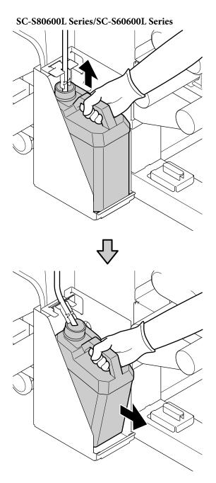
Insert the waste ink tube into the mouth of the new Waste Ink Bottle and place the Waste Ink Bottle in the holder.
