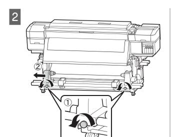
Align the roll core holder with the right edge of the media, and tighten the screw.
