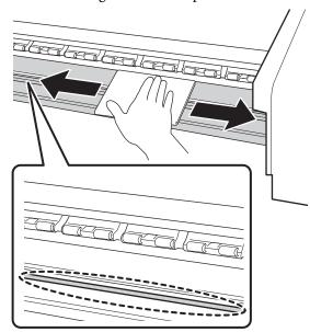
Soak a soft cloth in water, wring it out thoroughly, and then wipe off any lint, or dust that has adhered to the media edge plates.
