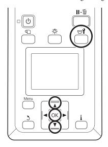
Confirm that the printer is on and press the 🗗 button.
