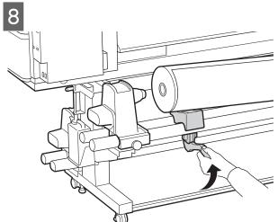
Firmly insert the roll core of the media onto the roll holder.
