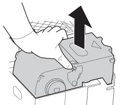
To avoid soiling your surroundings with ink, wrap the used wiper unit in the packaging supplied with the new wiper unit.
