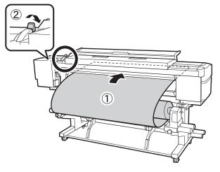
Confirm that the left edge of the media is within the range of the label's rectangle, as shown in the illustration below.
