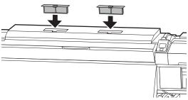
Check that the air filters are installed, and then press the OK button.
