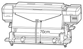
While pulling the paper tape straight down, wrap it around the roll core from back to front, and affix it using commercially available adhesive tape.
