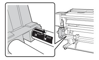
Tighten the screw until the screw no longer turns.
