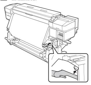
Hold the cutter vertically, and then move it so that the cutter blade fits closely to the side surface of the cutter groove.
