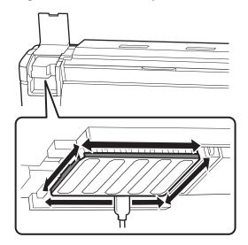
Wipe off any adhered ink, lint, and dust from the parts that are indicated by \_\_\_\_\_ below.
