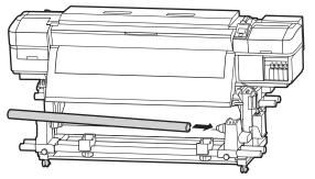
Push the holder until part A shown in the illustration below is fully inserted, and tighten the screw.
