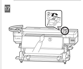
Hold the center of the media in one hand, and pull it straight until it is aligned with the bottom edge of the label on the after heater.
