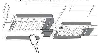
Wipe off any adhered ink, lint, and dust from the parts that are indicated by \_\_\_\_\_ below.
