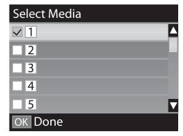
If media settings have not yet been made for new media, select an unassigned number, finish loading the media, and then perform Easy Media Setup.
