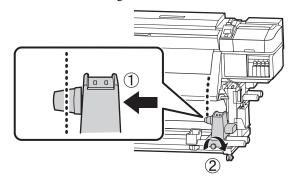
Insert the roll core onto the right holder.
