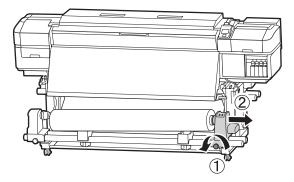
6 Lower the roll onto the roll support.
