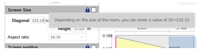
• Aspect ratio: The initial value is the aspect ratio of the LCD panel. When the aspect ratio setting is changed from the initial value, the black band will appear onto the left/right or top/bottom of the screen image.
