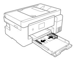
4. With the printable side facing down, load envelopes until it touches the back of the paper cassette.
