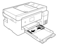
With the printable side facing down, load paper until it touches the back of the paper cassette.
