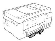
Check that the printer is not operating, and then slide out the paper cassette.
