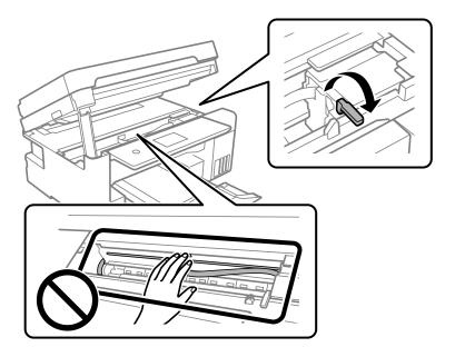
8. Secure the print head to the case with tape.
