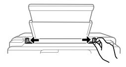
3. Load paper at the center of the paper support with the printable side facing up.
