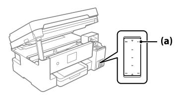
6. Align the top of the ink bottle with the filling port, and then insert it straight into the port to fill ink to the upper line.
