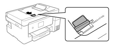
4. Place the originals face-up and short edge first in the ADF, and then slide the ADF edge guide to the edge of the originals.
