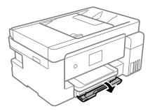
2. Check that the printer is not operating, and then slide out the paper cassette.
