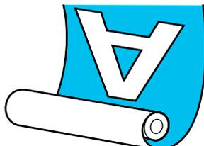
Taking-up with printed side out places the printed surface on the outside of the roll.
