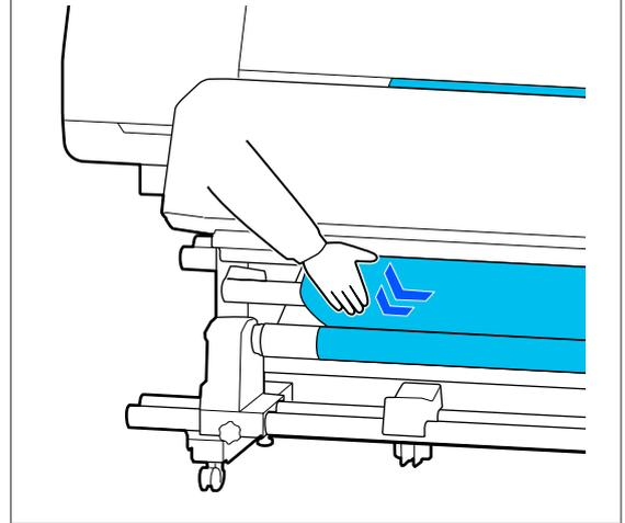
7 Continue holding down the
