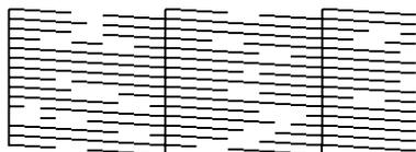
If there are gaps in the nozzle check pattern, press [X], and then perform Print Head Cleaning.
