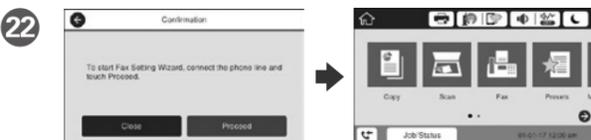
When the fax setting wizard screen is displayed, tap proceed to configure the minimum settings for fax features. If you do not setting now, close the fax setting screen. The home screen is displayed and printer is ready for printing.
