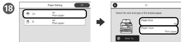
Check the paper size and paper type for the paper sources. Tap **OK** if the settings are correct, or select the correct paper size and paper type. You can change these settings later.
