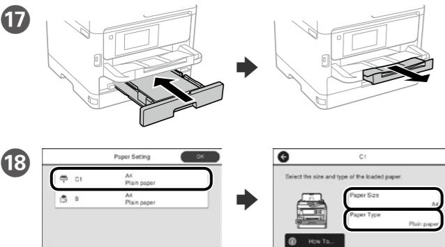
**17** Check the paper size and paper type for the paper sources. Tap **OK** if the settings are correct, or select the correct paper size and paper type. You can change these settings later.
