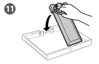
Fit the ink supply unit into the ink supply unit tray.
