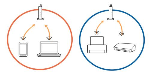
□ You may not be able to connect to the wireless router when the wireless router has multiple SSIDs and devices are connected to different SSIDs on the same wireless router. Connect the computer or smart device to the same SSID as the printer.
