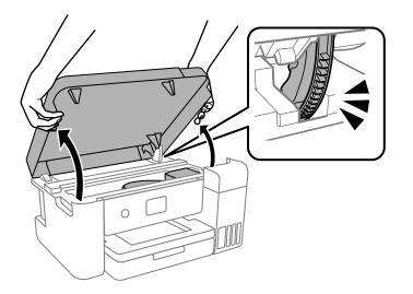
4. Check if the translucent film is smeared. Smears are easier to see if you use a light.If there are smears (such as finger marks or grease) on the translucent film (A), go to the next step.
