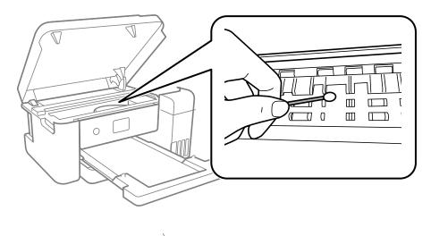
Do not touch the white flat cable, translucent film, and ink tubes inside the printer. Doing so may cause a malfunction.
