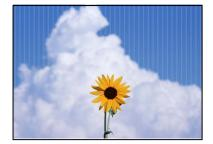
If you print using the standard quality setting, light banding may appear in the printout. When you transfer this to cloth, the banding may not be visible. Check the image after transfer. If banding appears even after transferring, print using a higher quality setting.
