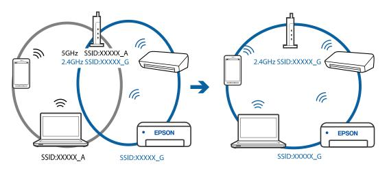
□ Most wireless routers have a privacy separator feature that blocks communication between connected devices. If you cannot communicate between the printer and the computer or smart device even if they are connected to the same network, disable the privacy separator on the wireless router. See the manual provided with the wireless router for details.
