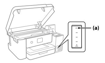
8. Align the top of the ink bottle with the filling port, and then insert it straight into the port to fill ink until it stops automatically at the upper line.
