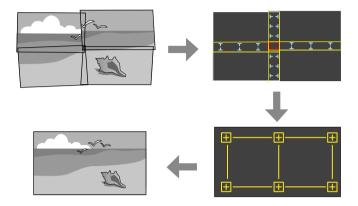
• Geometry Correction Assist - Stacking Function wizard allows you to easily and quickly create bright image by overlapping the images of multiple projectors. By adjusting the approximate size and position of your projected image, the projectors automatically overlap these images as one image.
