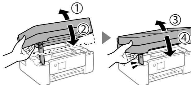
The unit must be closed completely before it can be opened again.
