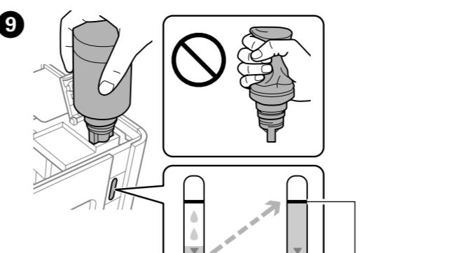
Ink flow stops automatically when the ink level reaches the upper line.
