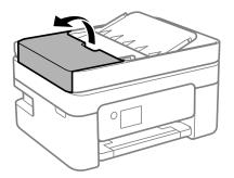
2. Use a soft, moist cloth to clean the roller and the interior of the ADF.
