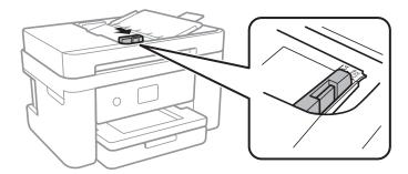
4. Place the originals face-up in the ADF, and then slide the ADF edge guide to the edge of the originals.
