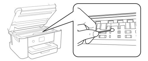
Do not touch the white flat cable and translucent film inside the printer. Doing so may cause a malfunction.
