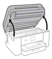
$^{3}\cdot\;\;$  Check if the translucent film is smeared. Smears are easier to see if you use a light. If there are smears (such as finger marks or grease) on the translucent film (A), go to the next step.
