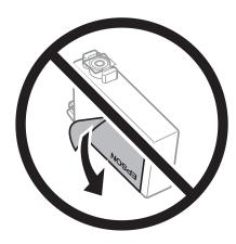
☐ Do not remove the transparent seal from the bottom of the cartridge; otherwise, the cartridge may become unusable.
