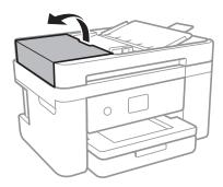
Use a soft, moist cloth to clean the roller and the interior of the ADF.
