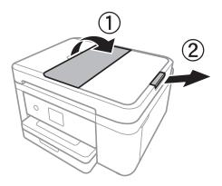
3. Pinch and slide out the ADF edge guide.
